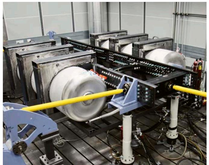
Meanwhile Boysen has tested the first prototype on a multi axis shaker concerning the mechanical load induced by road load. The quality of the insulation was determined through appropriate thermal loss tests.
